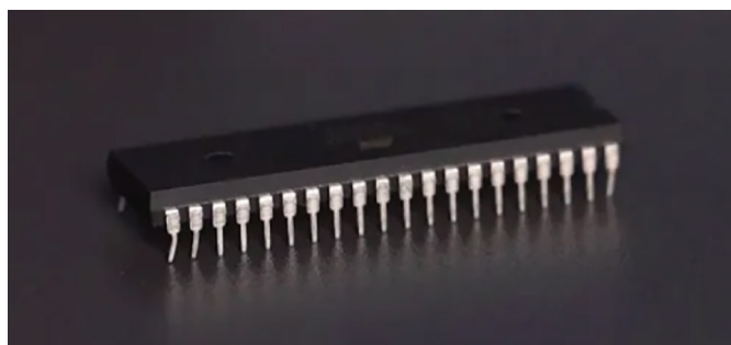
An 8-bit Atmega microcontroller from the first video of the 9th chapter of CCE1.
